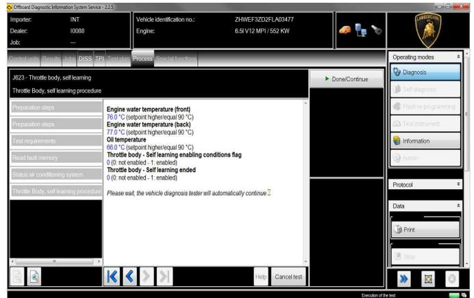
26. Once reached the activation conditions (water and oil temperatures major than 90°C) the “Throttle body – Self learning enabling con-ditions flag” changes from 0 to 1 indicating the start of the self-learning procedure.
