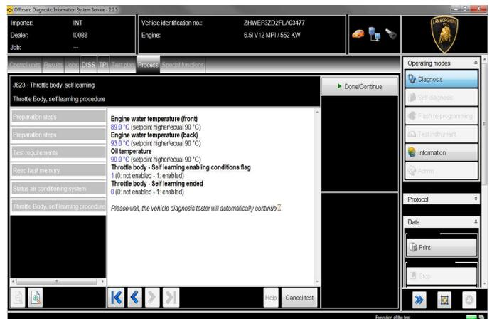
27. If the self-learning is completed successfully a screen as in the picture below is shown.
