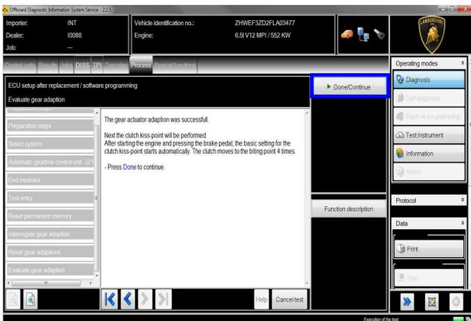
**12. Start the engine at idle and keep pressed the brake pedal for at least 1 minute.**
